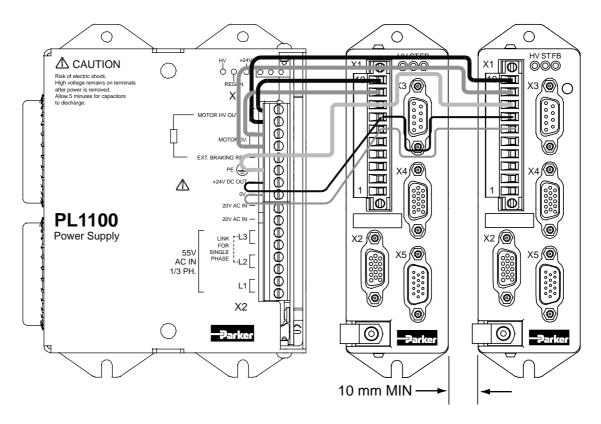
Figure 3-4. PL1100 Power Supply and Drive Connections
